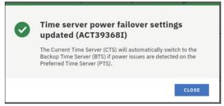
Figure 3-44 Confirmation message: N-mode power failover for the PTS has been enabled
