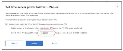
Figure 3-42 Failback timer (BTS -> PTS after N-mode switch on PTS)
